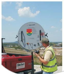
The Long Range Acoustic Device (LRAD) represents the new generation of wildlife control devices. The LRAD system is capable of providing controlled delivery of bioacoustics at variable volumes in a tight beam at ranges to 1000 meters. LRAD for bird and wildlife control is supported by DeTect, the industry leader in airfield wildlife control and detection technologies and systems.
